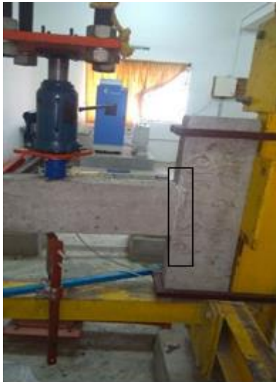
Fig 5: Cracks observed in specimen with Stirrups spacing -100 mm
