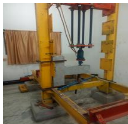
FIG 4: LOADING FRAME & HYDRAULIC JACK ATTACHED TO SPECIMEN
