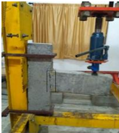
Fig 6: Cracks observed in specimen with 70mm stirrups spacing
